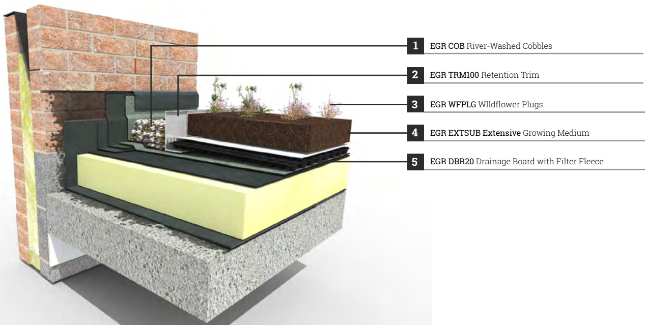
The diagram is for illustration only. The waterproofing membrane demonstrates just one example of applicable detailing.
