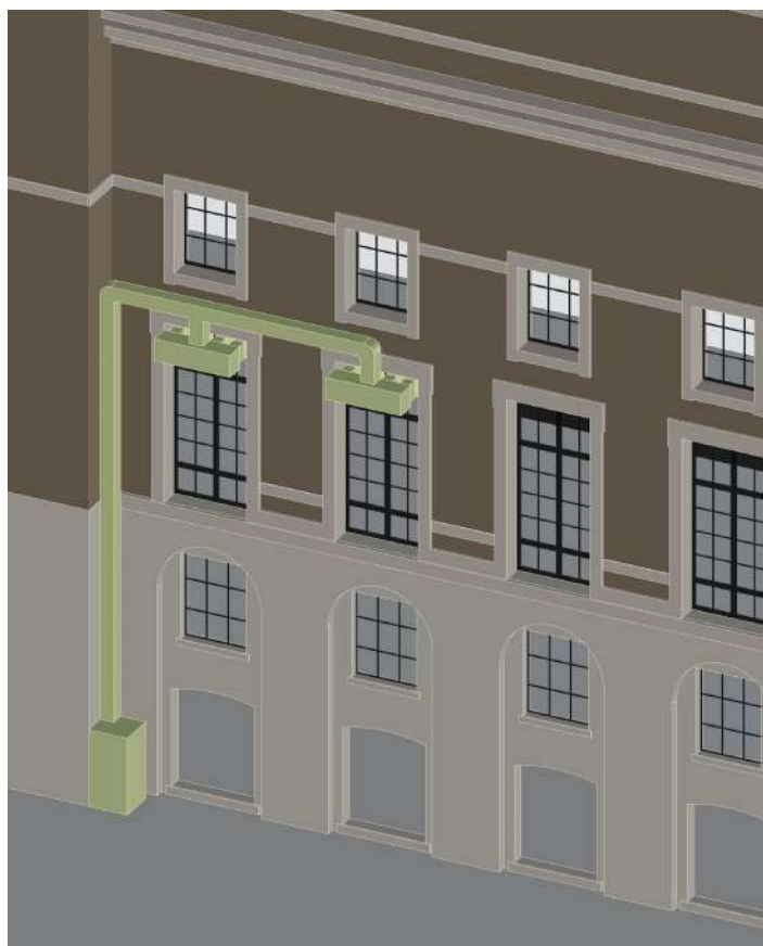
Proposed new ducting and extract fan unit in the bottom corner
