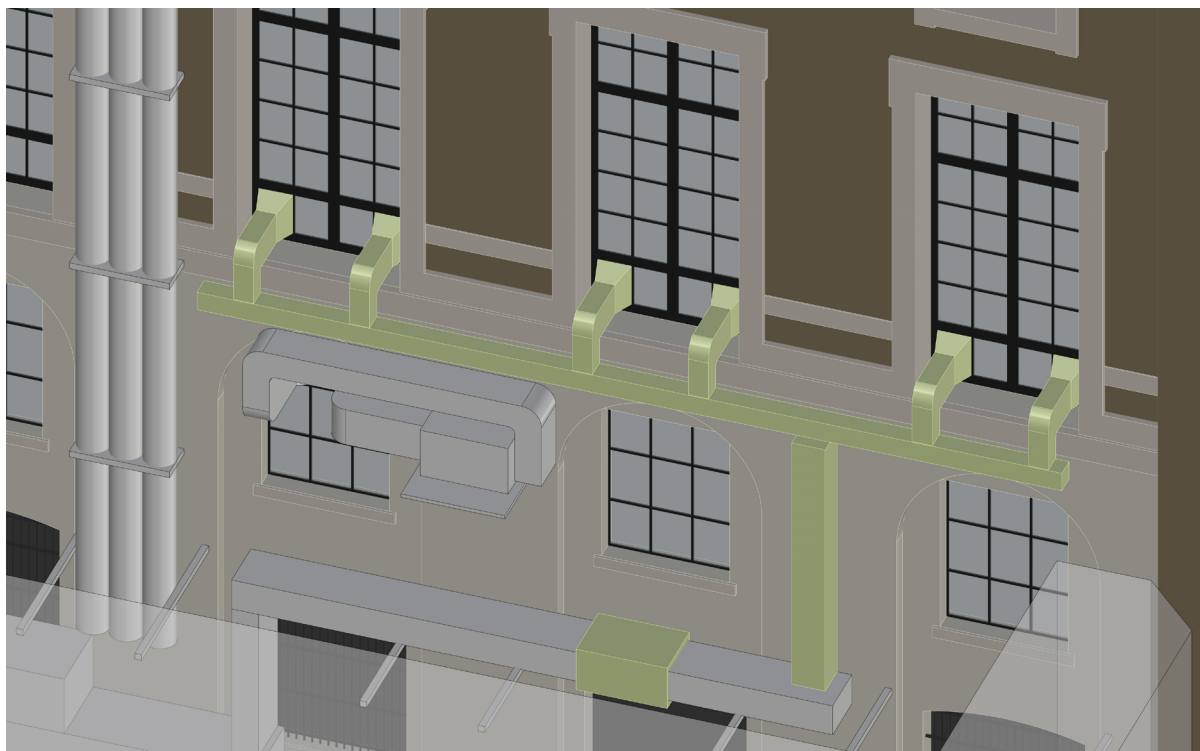
Image of proposed additional ducting in green. Existing ducting is shown in grey.
