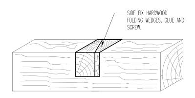
NOTCH REPAIR DETAIL 2
