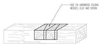
NOTCH REPAIR DETAIL FOR LONG NOTCH
