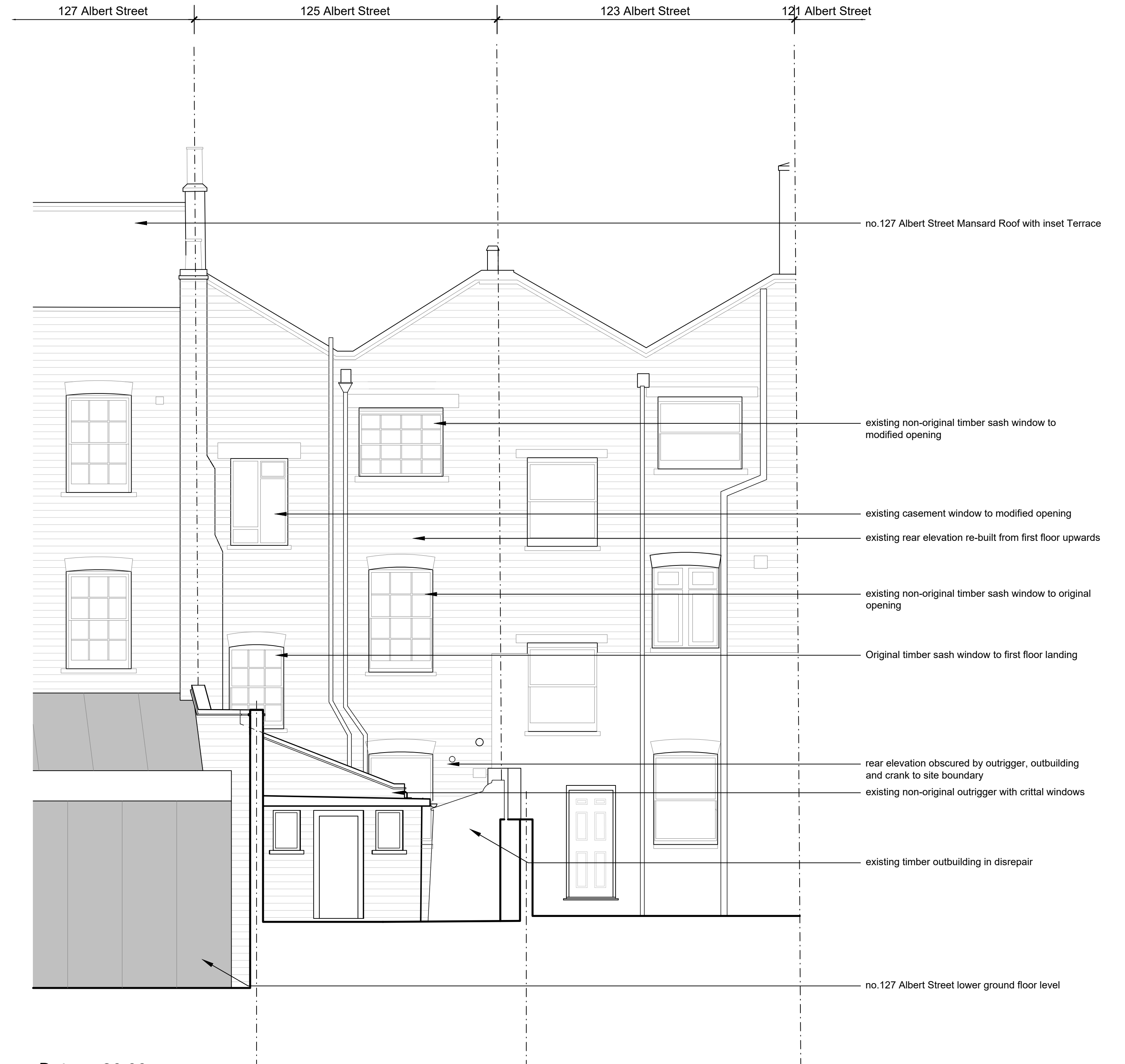
02 Existing Rear Elevation EX-2.00
