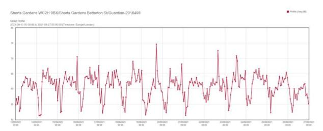
The graph below shows a typical daily Dust or air quality reading. Above the graph is the unit identification and to the right is the graph legend. The legend represents the different sizes of particulate mass. (PM10, PM2.5 & PM1) Most local authorities are interested purely in PM10 levels, for construction projects, and this is represented by the green line on this graph. Samples are analysed over a 15-minute period and the result is the level shown.
