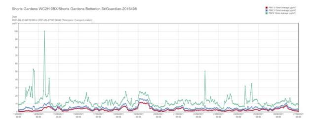
The graph below shows a typical daily vibration reading. Above the graph is the unit identification and to the right is the graph legend. The ambient levels shown are very low and we would expect to see levels averaged over a working day at around 2mm/s based purely on pedestrian activity. Add traffic activity and we would expect to see averages around 4mm/s
