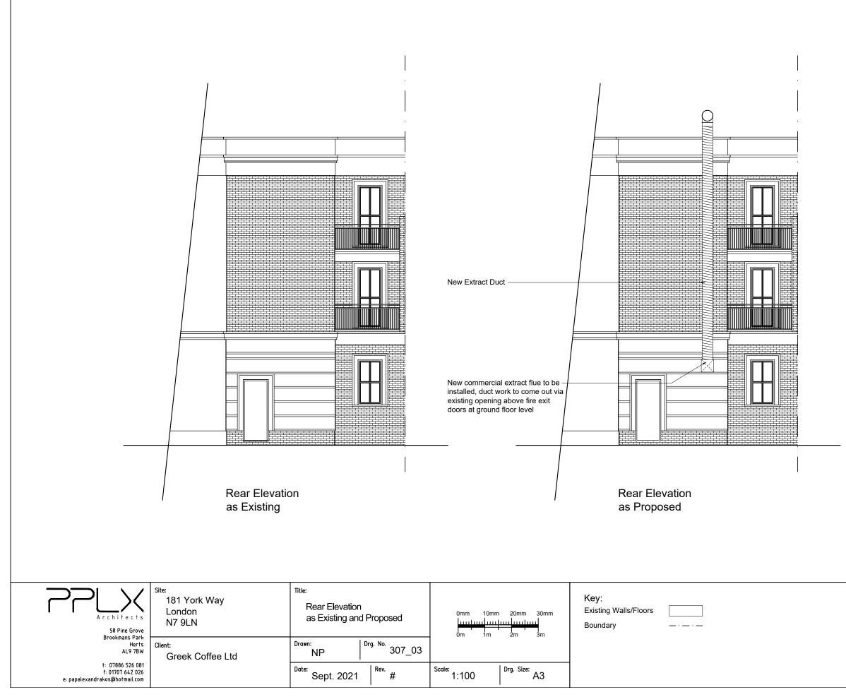
Stack height to be a miniumum of 1m above roof eaves, to ensure adequate dilution of odours to take place before the plume interacts with a receptor.
