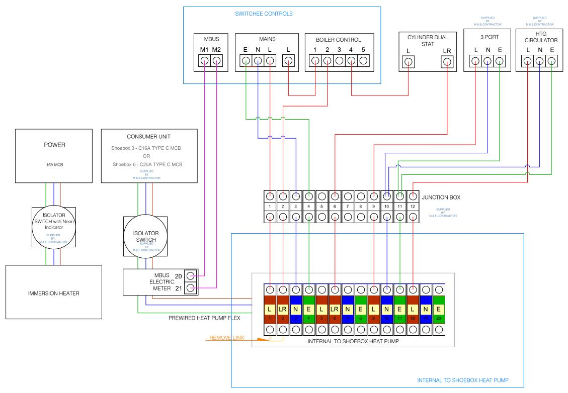
Control wires from heat pump to junction box should be a single multi-core cable
