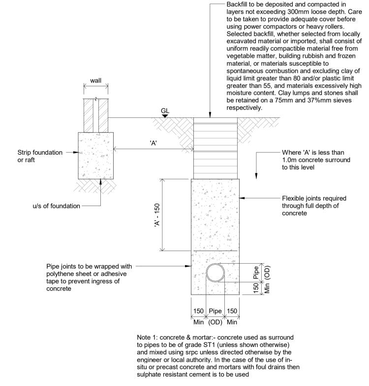
NOTE: NOT APPLICABLE TO PILED AND BEAM FOUNDATIONS
