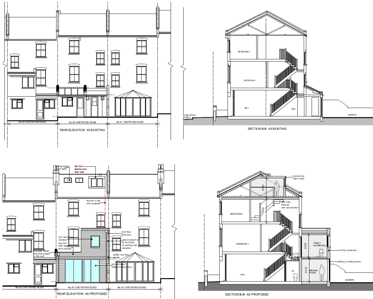
Figure 2 - Existing (Top) and Proposed (Bottom) Elevations and Sections
