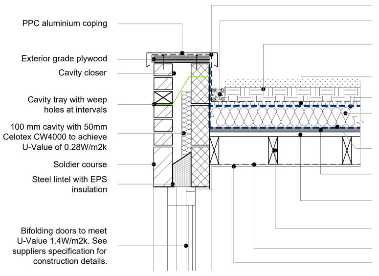
Single ply waterproof membrane Pebble ballast/gutter about perimeter.
