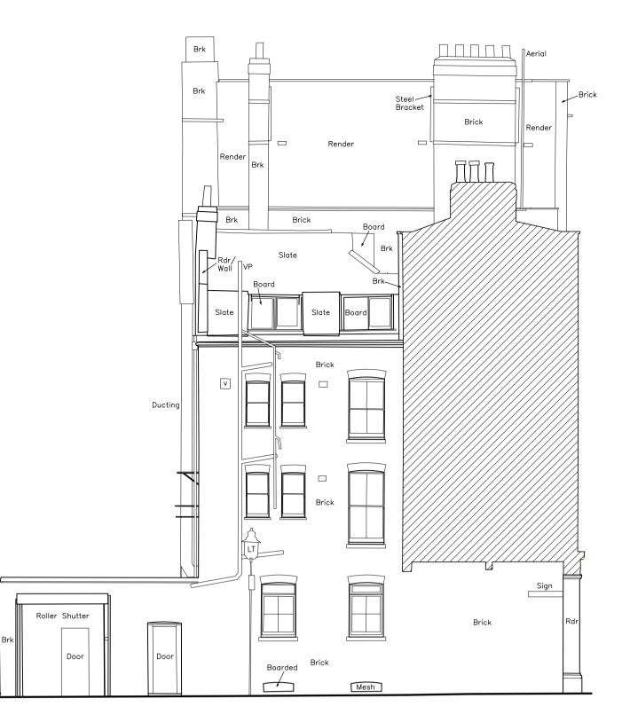
Proposed Side (South) Elevation (Unchanged) Scale 1:100
