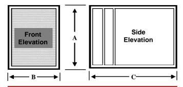
Minimum Carbon Weight Loading: 80 kg/1.0m³/sec Resistance to airflow: 175 Pa excluding prefilter and grease filter
