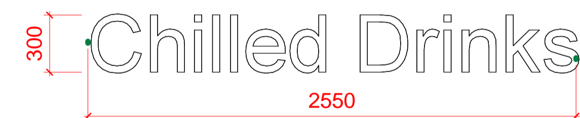
SIGN 5 1 : 20 INTERNAL SIGN CHILLED DRINKS LED FACE ILLUMINATED SIGNAGE MOUNTED CENTRALLY ONTO BULKHEAD FASCIA.
