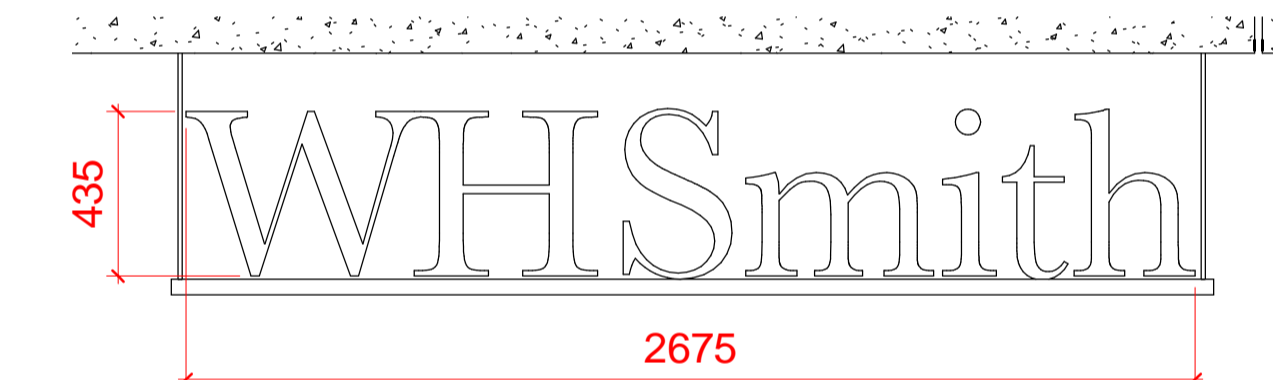
SIGN 4 1 : 20 WHS LED FACE ILLUMINATED SIGNAGE MOUNTED ON 40MM SHS BAR HUNG FROM SUITABLE POINT IN LINE WITH SE DETAILS
