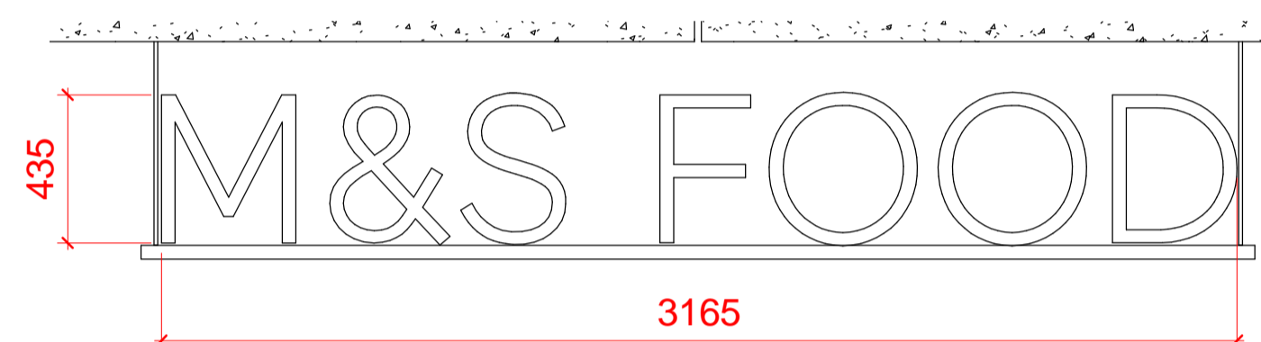
SIGN 3 1 : 20 M&S FOOD LED FACE ILLUMINATED SIGNAGE MOUNTED ON 40MM SHS BAR HUNG FROM SUITABLE POINT IN LINE WITH SE DETAILS
