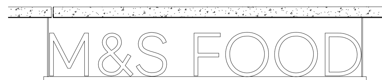
SIGN 2 1 : 20 M&S FOOD LED FACE ILLUMINATED SIGNAGE MOUNTED ON 40MM SHS BAR HUNG FROM SUITABLE POINT IN LINE WITH SE DETAILS
