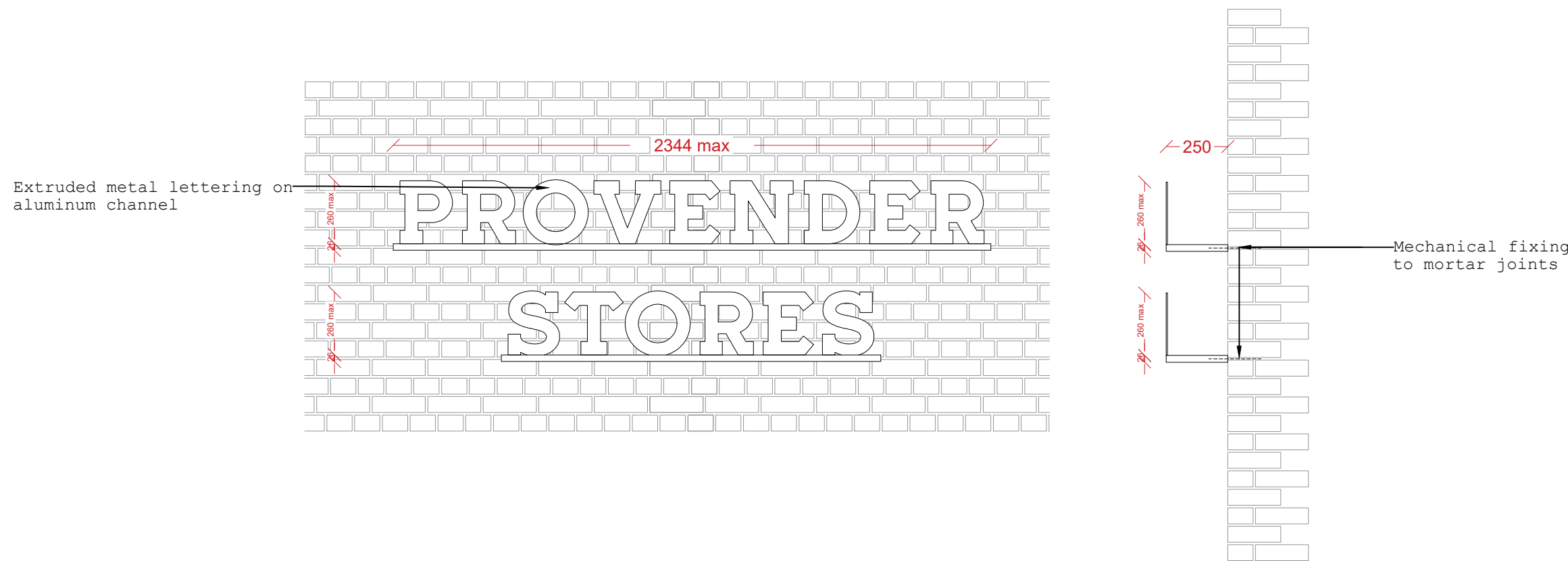
02 EXT 3 SIGNAGE HERITAGE FIXING DETAIL SCALE 1:20 © A1
