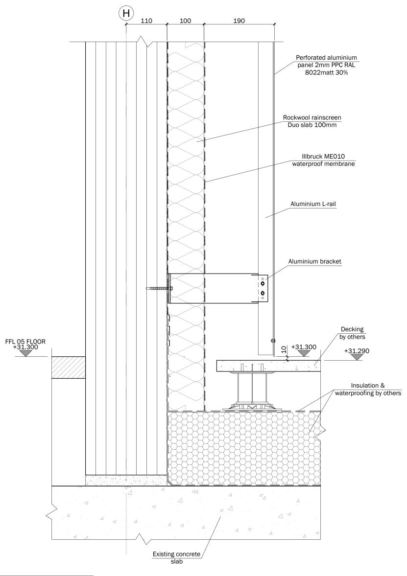
All penetrations in Illbruck membrane to be sealed in accordance with waterproofing specialist's details. Detail between window frame and membrane as per manufacturer's requirements
