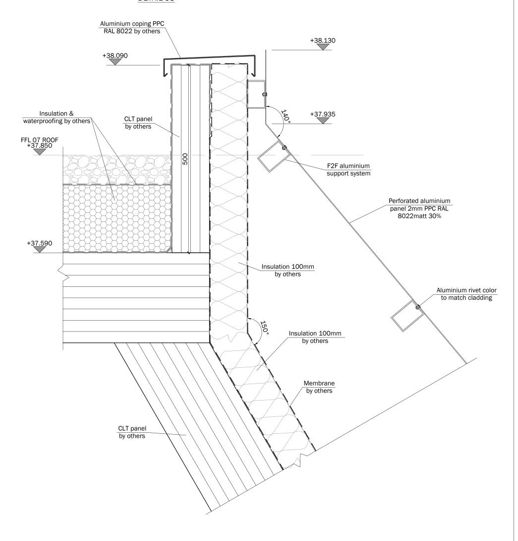
All penetrations in Illbruck membrane to be sealed in accordance with waterproofing specialist's details. Detail between window frame and membrane as per manufacturer's requirements
