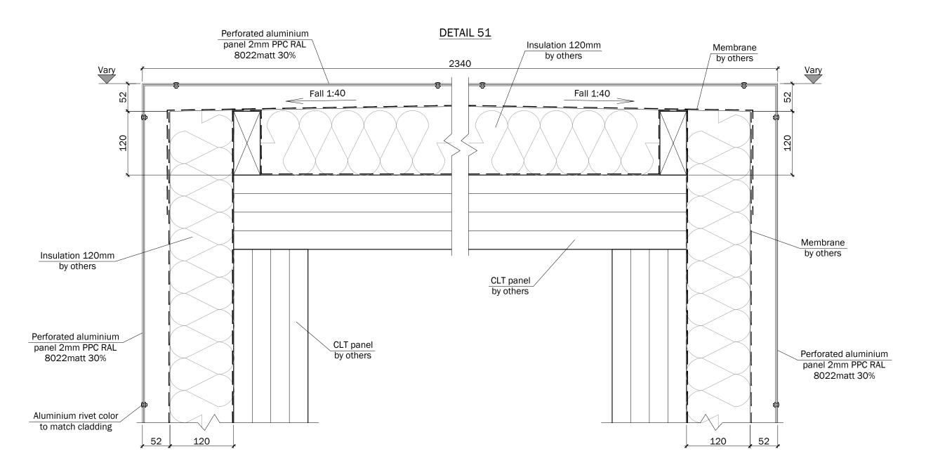
All penetrations in Illbruck membrane to be sealed in accordance with waterproofing specialist's details. Detail between window frame and membrane as per manufacturer's requirements
