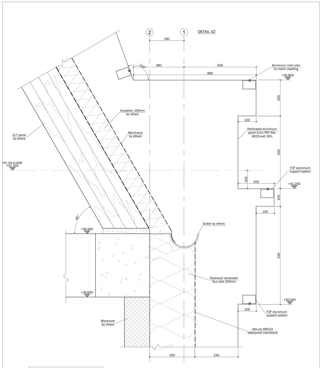
All penetrations in Illbruck membrane to be sealed in accordance with waterproofing specialist's details. Detail between window frame and membrane as per manufacturer's requirements
