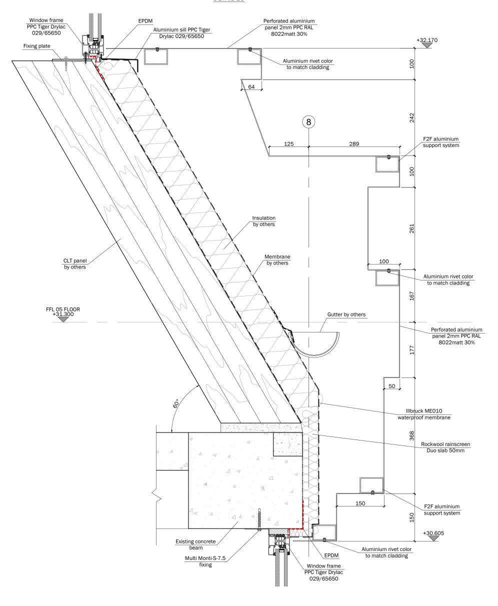
All penetrations in Illbruck membrane to be sealed in accordance with waterproofing specialist's details. Detail between window frame and membrane as per manufacturer's requirements
