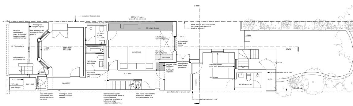
Delta membrane or approved other waterproofing system to all walls and floors in lower ground / basement level • underfloor heating throughout lower ground floo
