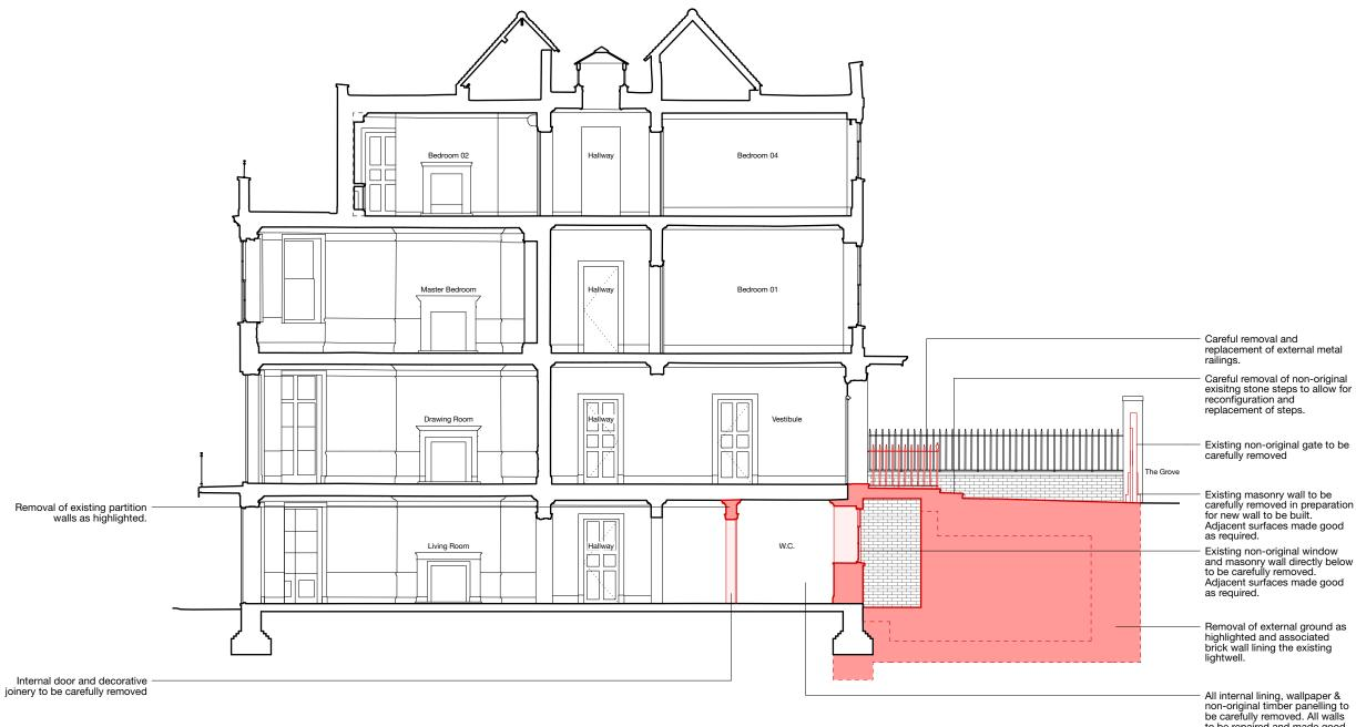
All internal lining, wallpaper & non-original timber panelling to be carefully removed. All walls to be repaired and made good. Walls to be plastered with skim coat finish prior to re decoration re-decoration.
