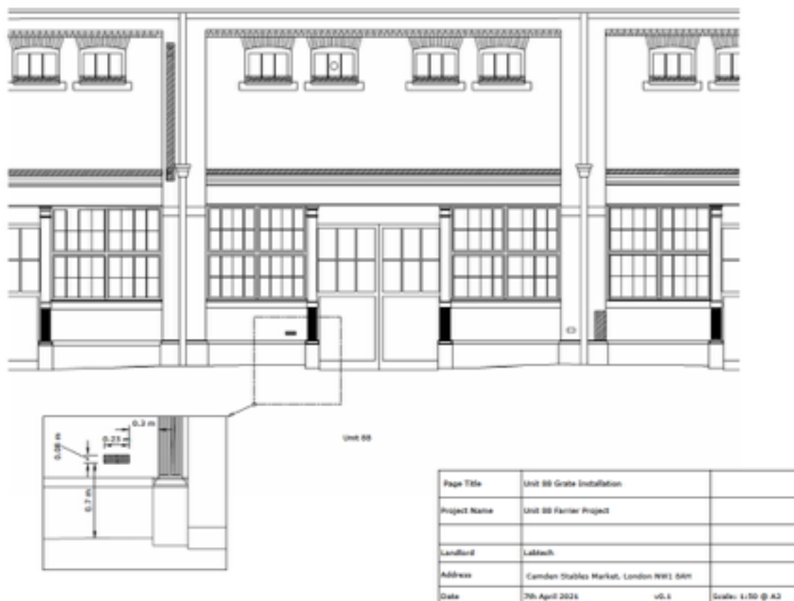
Figure 6: Front elevation of unit 88 of the Horse Hospital where grille is to be installed.
