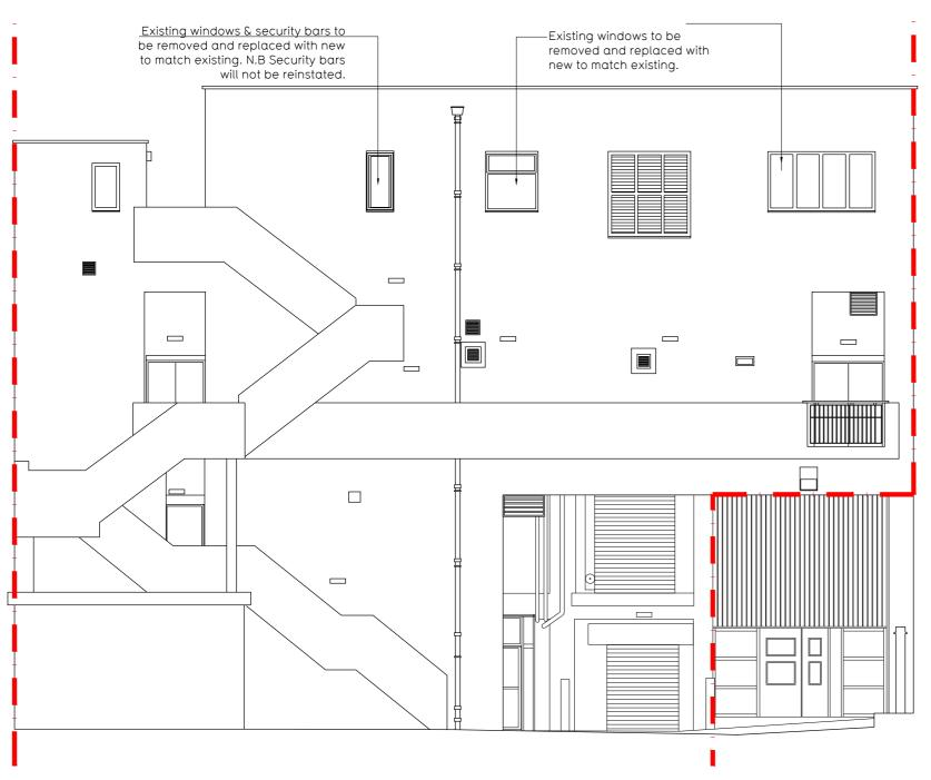
Elevation A Proposed Rear Elevation - 1:100
