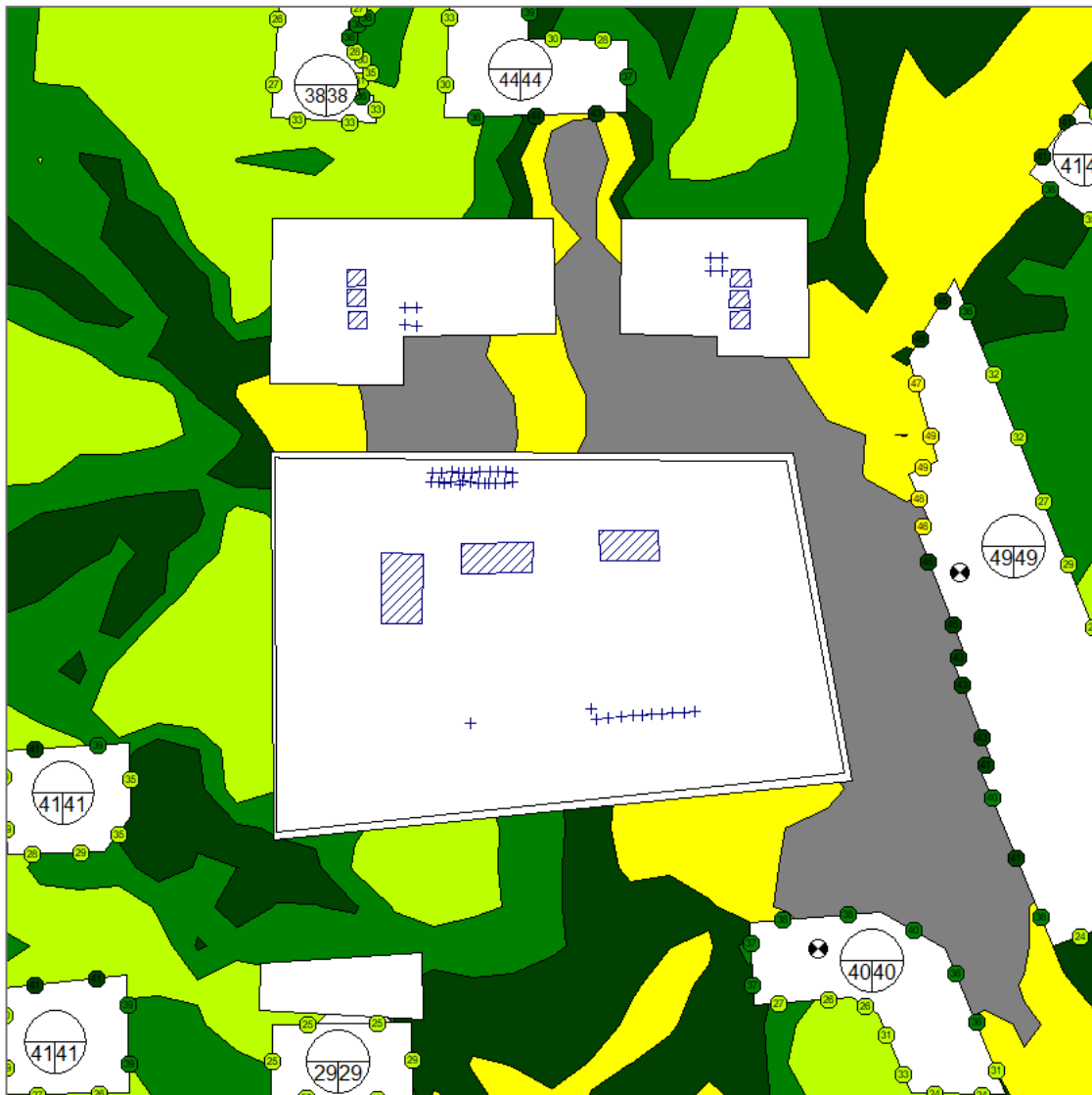
CadnaA model showing noise levels expected at nearest noise sensitive facades during daytime (2D view)
