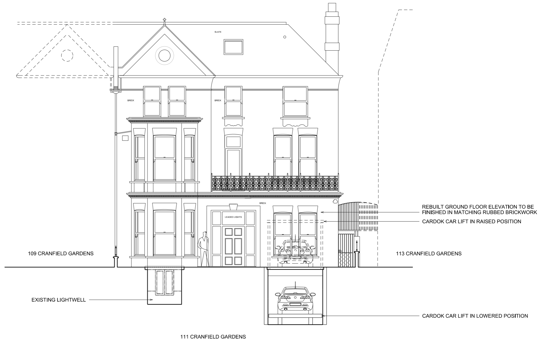
PROPOSED CRANFIELD GARDENS (FRONT) ELEVATION AND SECTION THROUGH BASEMENT CAR LIFT & EXISTING BEDROOM LIGHTWELL
