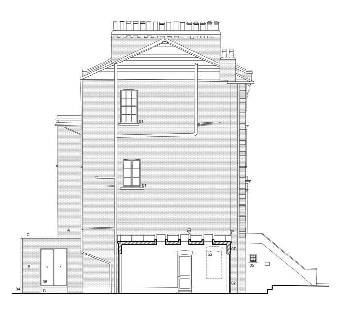
Side extension pushed back by approximately 800mm from front facade for subervience. The new position aligns with existing wall detail and is set in front of the existing side window. 07
