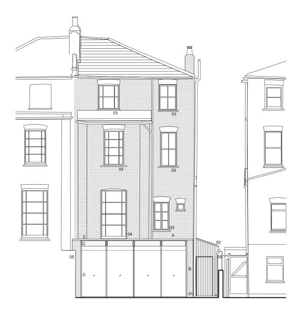
Section of wall re-built in brick to match existing. 05 Wall raised in line with extensions. Please refer to elevations.
