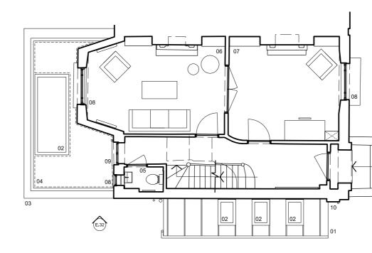
10 Side extension pushed back by approximately 800mm from front facade for subervience. The new position aligns with existing wall detail and is set in front of the existing side window.
