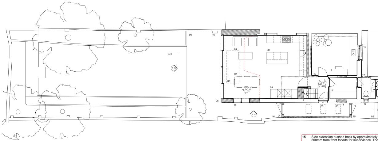
800mm from front facade for subervience. The new position aligns with existing wall detail and is set in front of the existing side window. Section of wall re-built in brick to match existing. Wall raised in line with extensions. Please refer to elevations.
