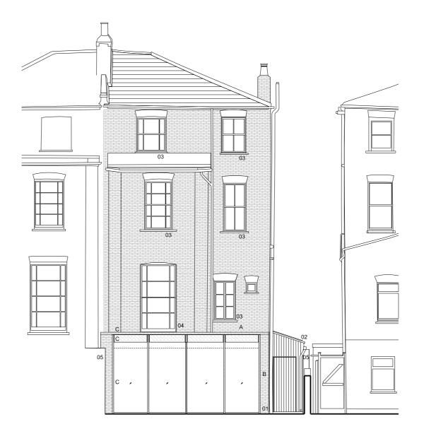
Section of wall re-built in brick to match existing. Wall raised in line with extensions and raised to height of 1.7m opposite the new side windows to the extension.
