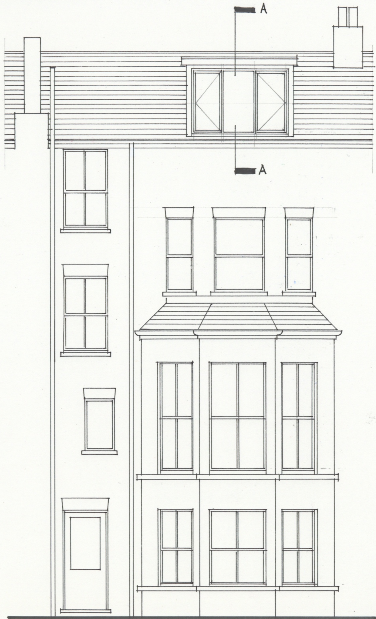
PROPOSED REAR ELEVATION. SCALE: 1:50 @ A3.
