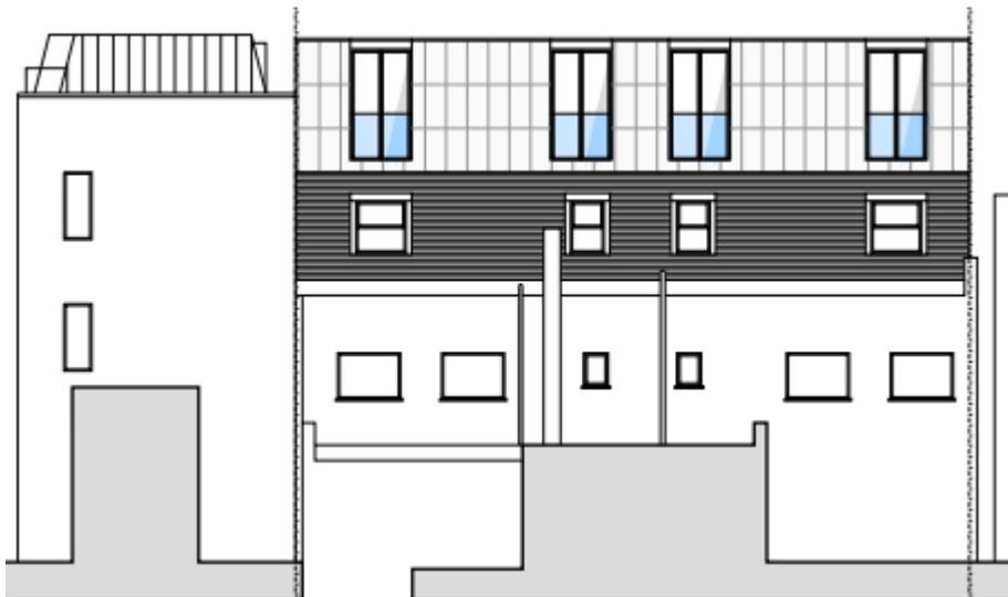
8.6 The area of the windows shaded in blue are designed to be fixed shut and obscure glazed to ensure no overlooking into neighbouring windows.
