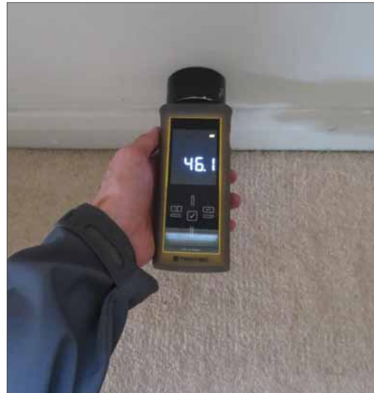
Images 41 & 42: High External Ground Levels to North West Corner of the House & Corresponding Elevated Masonry Moisture Reading.
