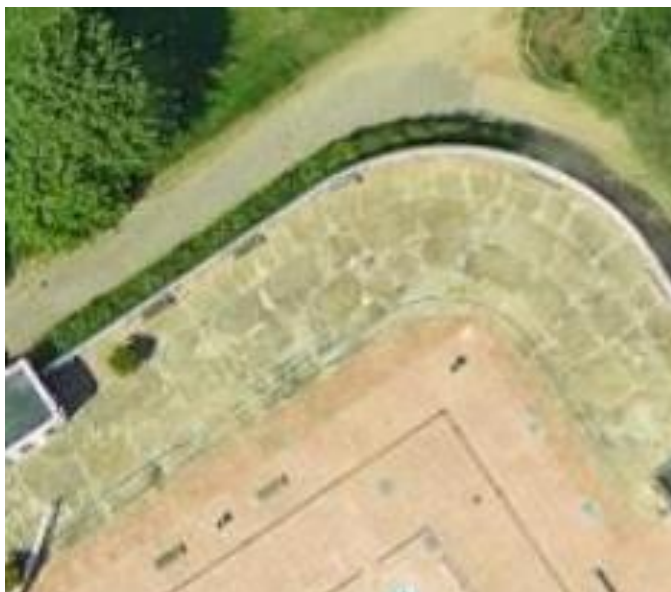
Aerial detail (left) and terrace image showing self-determined cracking occurring at approximately 2 to 2.5 m centres
