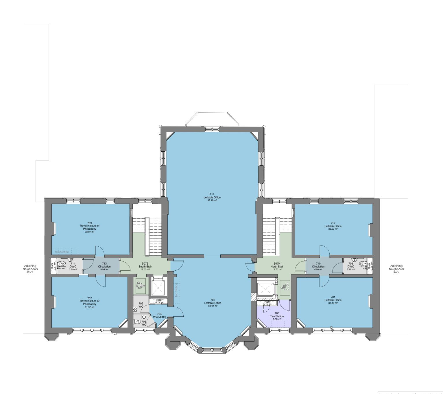
Wall Colour Key Existing Fabric- Shown in grey Circulation (Letting) Circulation (shared) Existing Fabric- Doors to be retained and locked shut. Office (Letting) New Construction- Shown in white Adjoining properties, highlighted by cross hatch- shown indicatively to provide context. Tea Station
