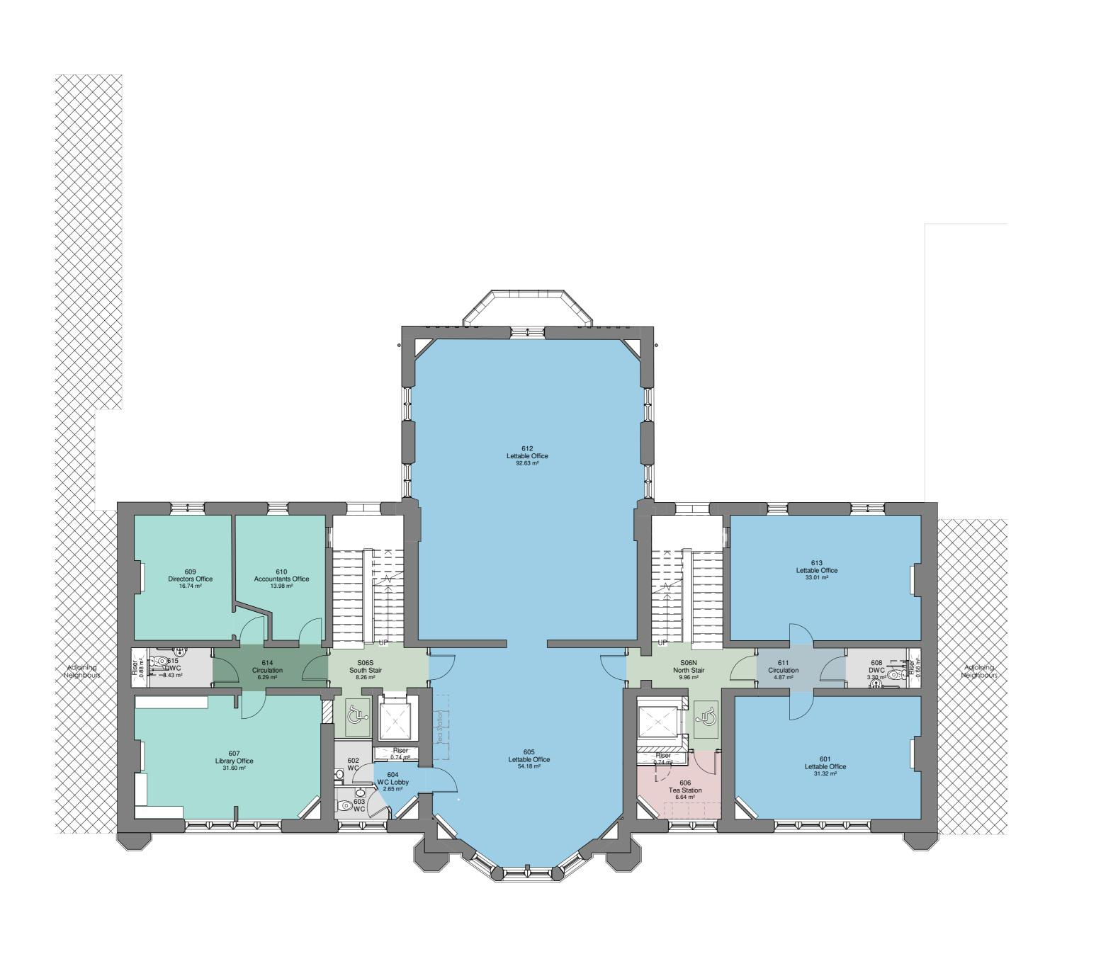
Wall Colour Key Existing Fabric- Shown in grey Circulation (Letting) Existing Fabric- Doors to be retained and locked shut. Circulation (Library) New Construction- Shown in white Circulation (shared) Adjoining properties, highlighted by cross hatch- shown indicatively to provide context.
