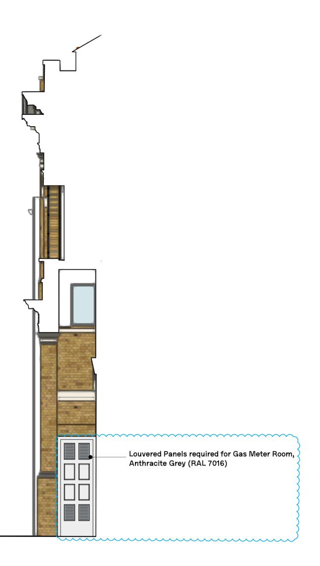
Elevation: East Elevation of Entrance Portico Scale: 1:50
