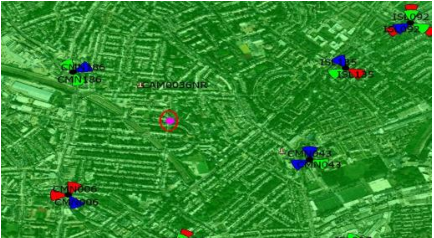
Figure 5: Cell Search Area Map with the Nominal illustrated by the pink dot.
