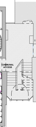
NEW METAL BALUSTRADE BEHIND EXISTING MASONRY BALUSTRADE
