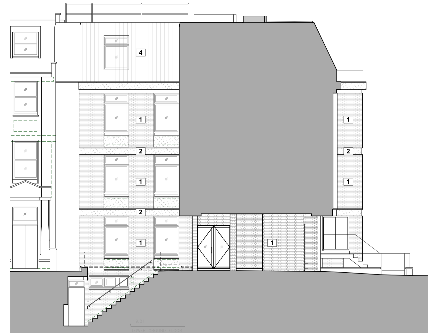
3 Elevation 05 Entrance to west building moved, appearance to match existing Addition of lift overrun 1:100
