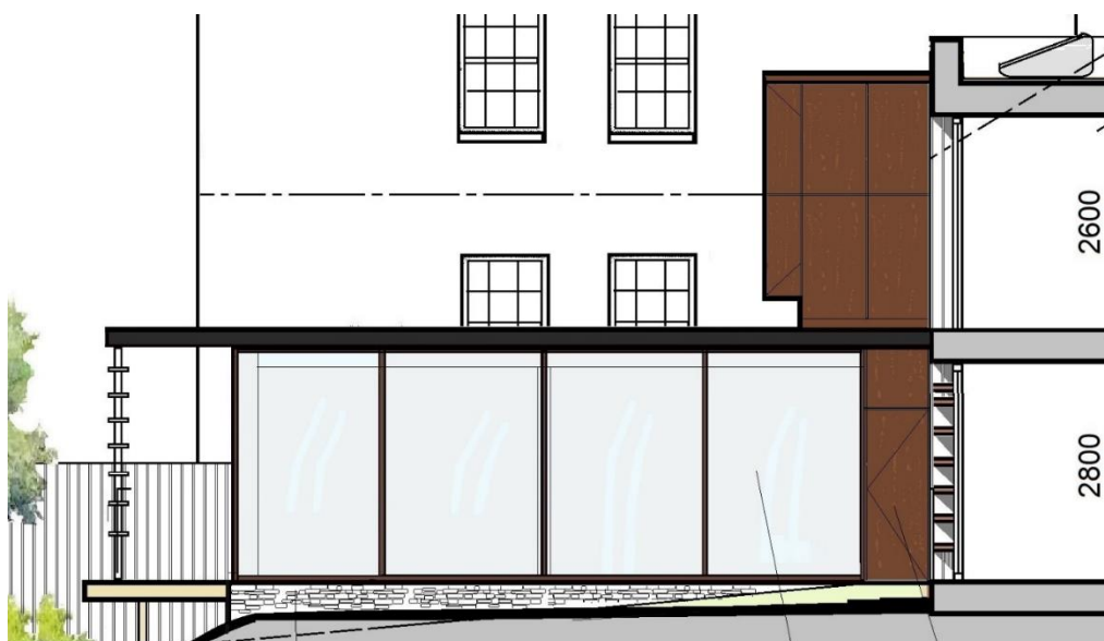
SECTION SHOWING TIMBER LOUVERS TO ACT AS SOLAR SHADING AND PRIVACY SCREEN
