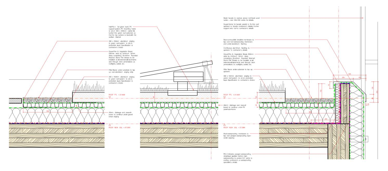
(1) GREEN ROOF TO CONCRETE PAVING SLAB DETAIL
