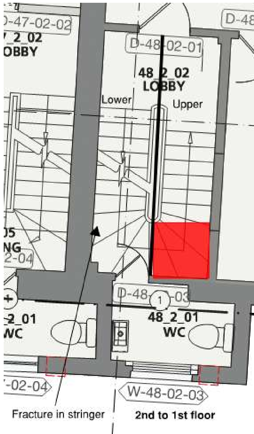
Fig.2 2 nd to 1 st floor upper and lower flights highlighted with fungal decay.
