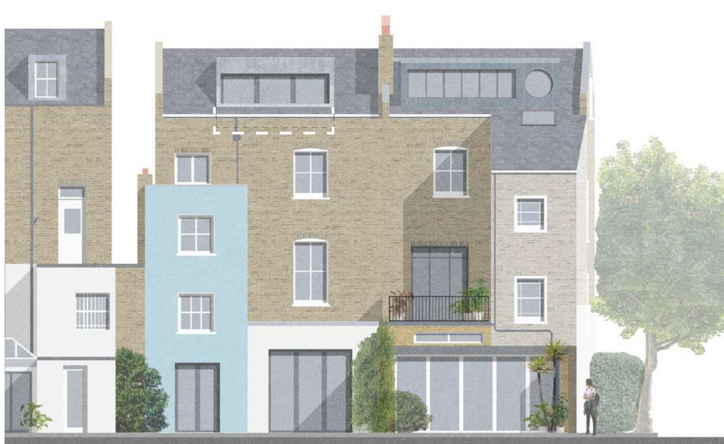
Rear elevation showing proposed dormer and outrigger roof works
