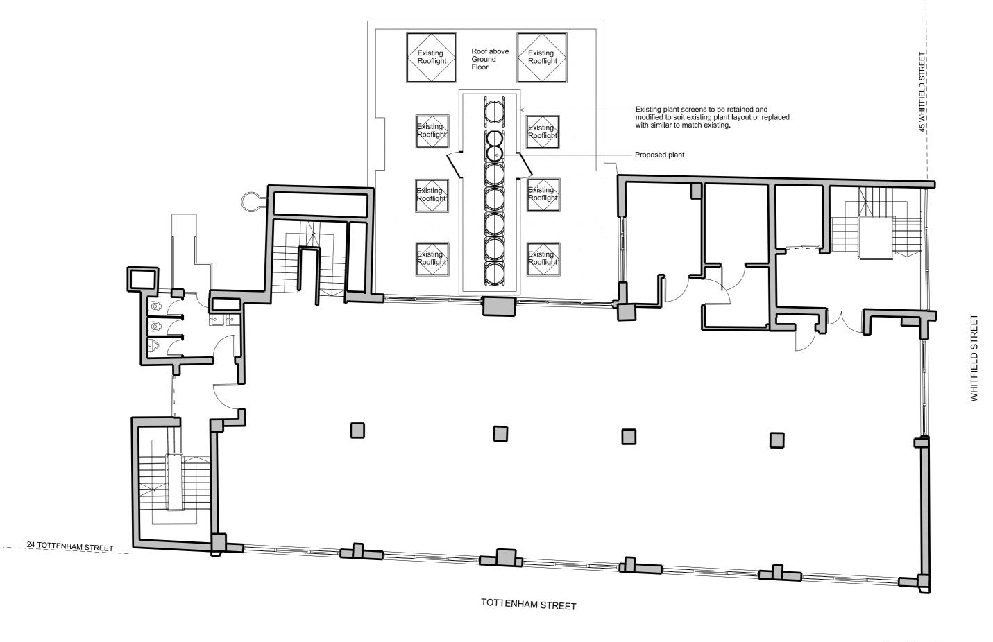
06/08/2021 09/06/2021 Date FeildenCleggBradleyStudios LLP Job/Drawlng No 2052/015 Amendment P02 43 WHITFIELD STREET, W1T 4HD PROPOSED FIRST FLOOR PLAN AND PROPOSED PLANT LAYOUT TO GROUND FLOOR ROOF Scale 1:100 @ A3
