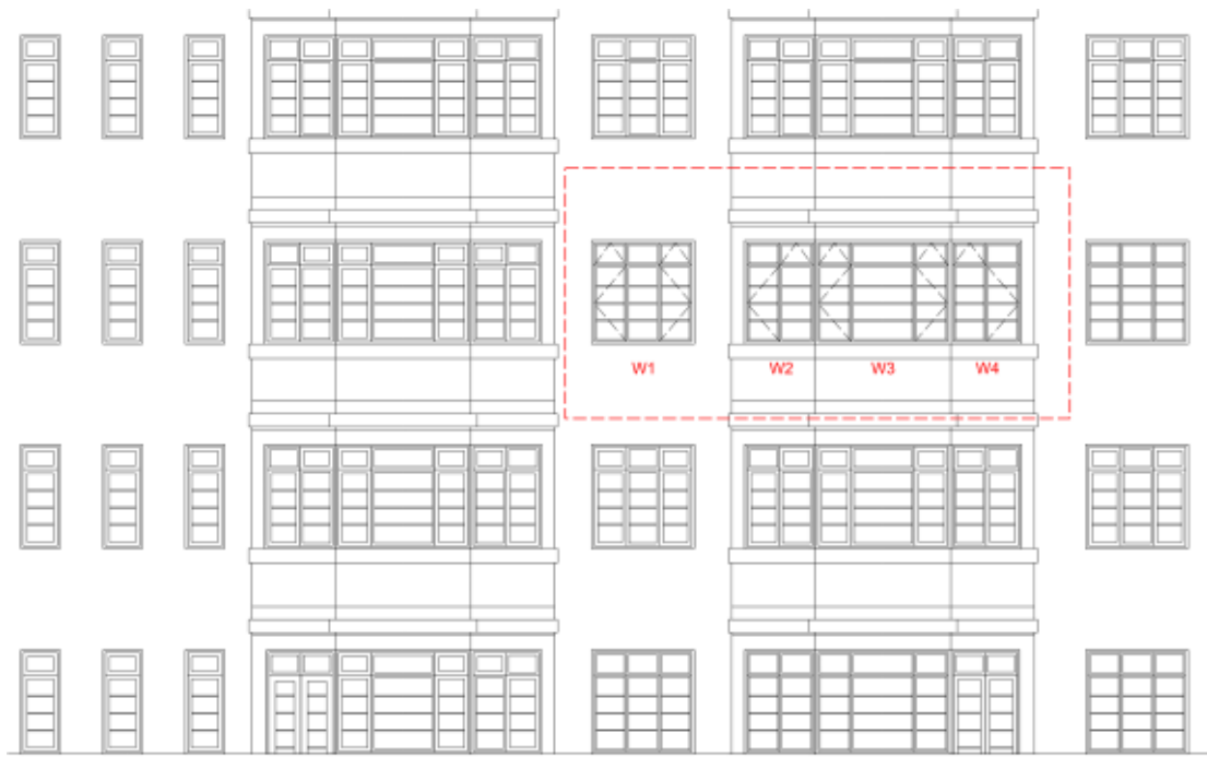
View 3 – existing south-west elevation showing 4 windows to be replaced
