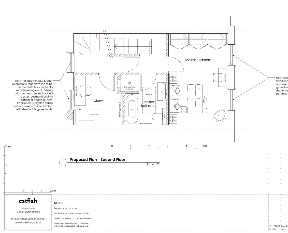
New sash windows as required to building to be traditionally weighted vertical sliding sash windows in painted timber with slim double glazed units. Existing timberwork - architraves, shutters etc. - to interior to be salvaged if possible.
