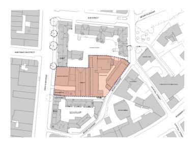
Redevelopment of existing buildings to provide part 4 storey and part 7 storey building following partial demolition of existing Panther House and Brain Yard buildings for a mix of Class B1, A1 and A3 uses, provision of new 7 storey building at 156-164 Gray's Inn Road behind the facade from existing building at 160-164 Gray's Inn Road to provide flexible Class A1 use at ground and basement levels and 13 self-contained residential units (4 x 1-bed, 7 x 2-bed and 2 x 3-bed) at upper floor levels."
