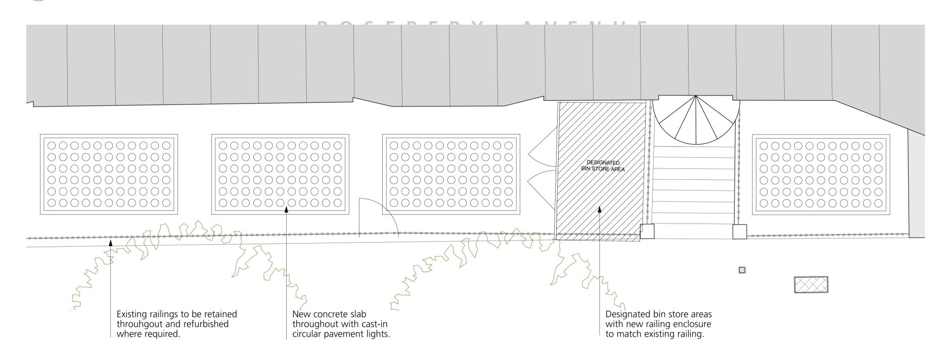
Proposed Plan - Pavement Lights Scale: 1:50
