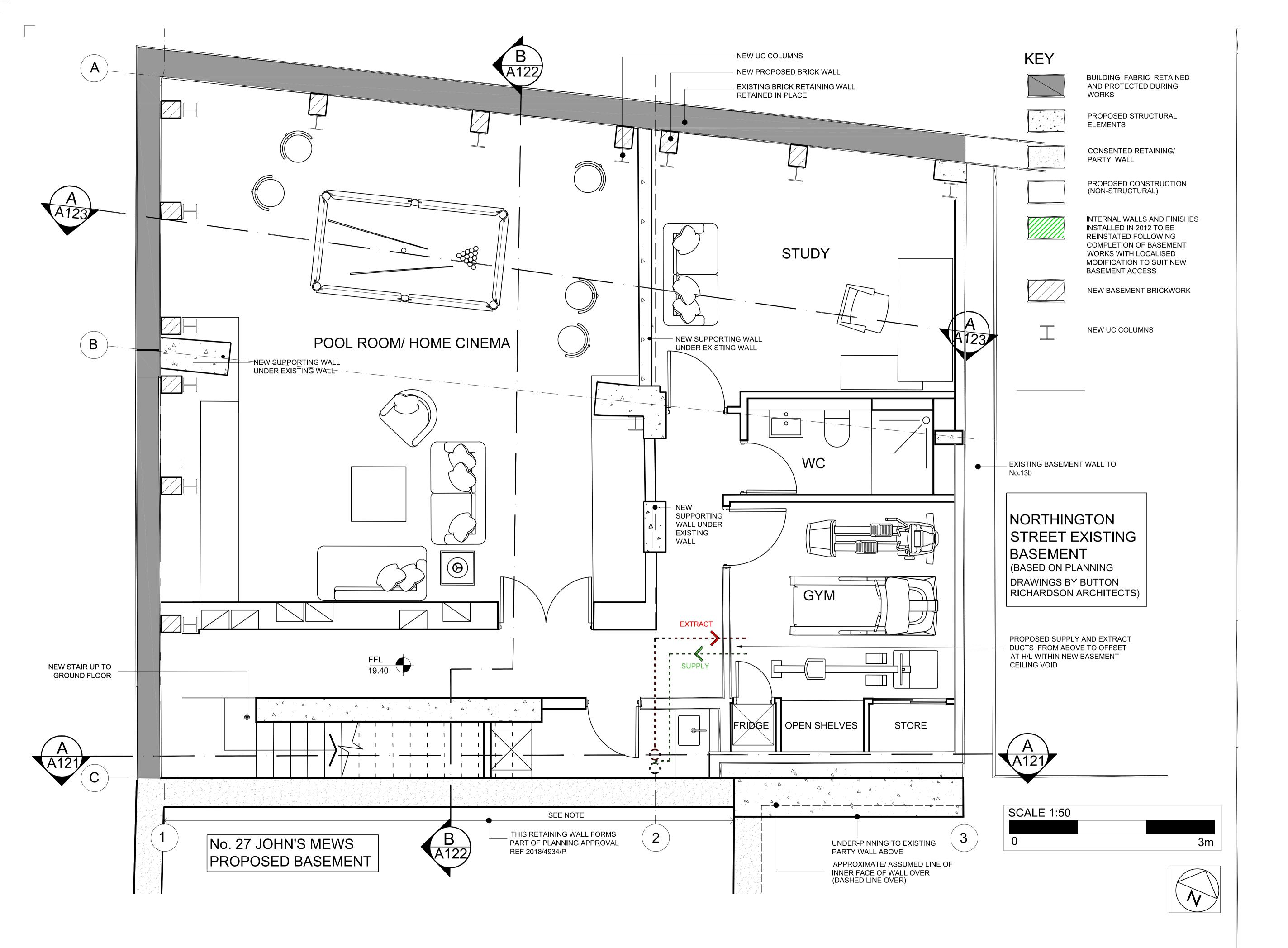
D 06.08.21 DELETED COVERING BRICKWALLS JC / CD C 30.06.21 REVISED NEW PLANNING DRAWING JC / CD SHOWING NEW UC AND BASEMENT BRICK WALLS TO SUPPORT EXISTING WALLS ON GROUND FLOOR
