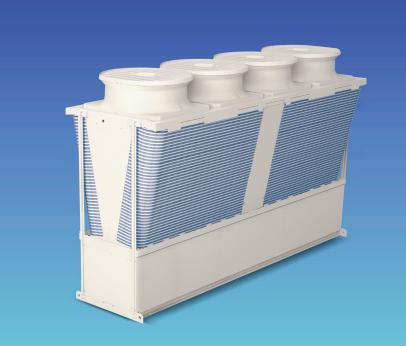
The **e-series chiller** allows for up to six individual units to be connected together to provide a system capacity from 90kW to 1,080kW. Using this modular approach reduces space requirements and simplifies lifting and installation. The e-series chiller is available as a cooling only or heat pump version, suitable for both comfort and process cooling applications.
