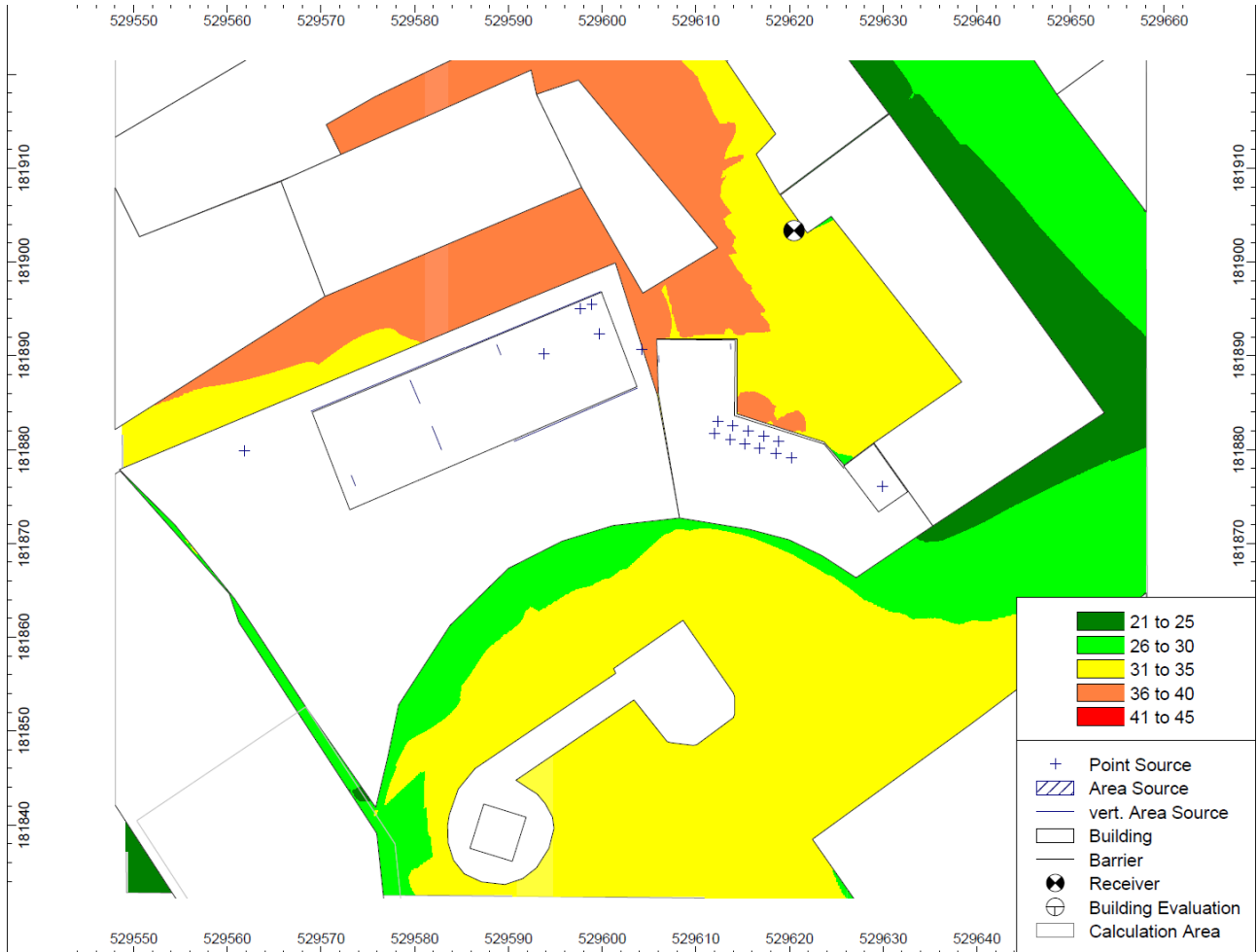
Figure E.3 2D Noise Contours Map showing specific plant noise level L_{Aeq} , dB at the height of top windows of the residential buildings.
