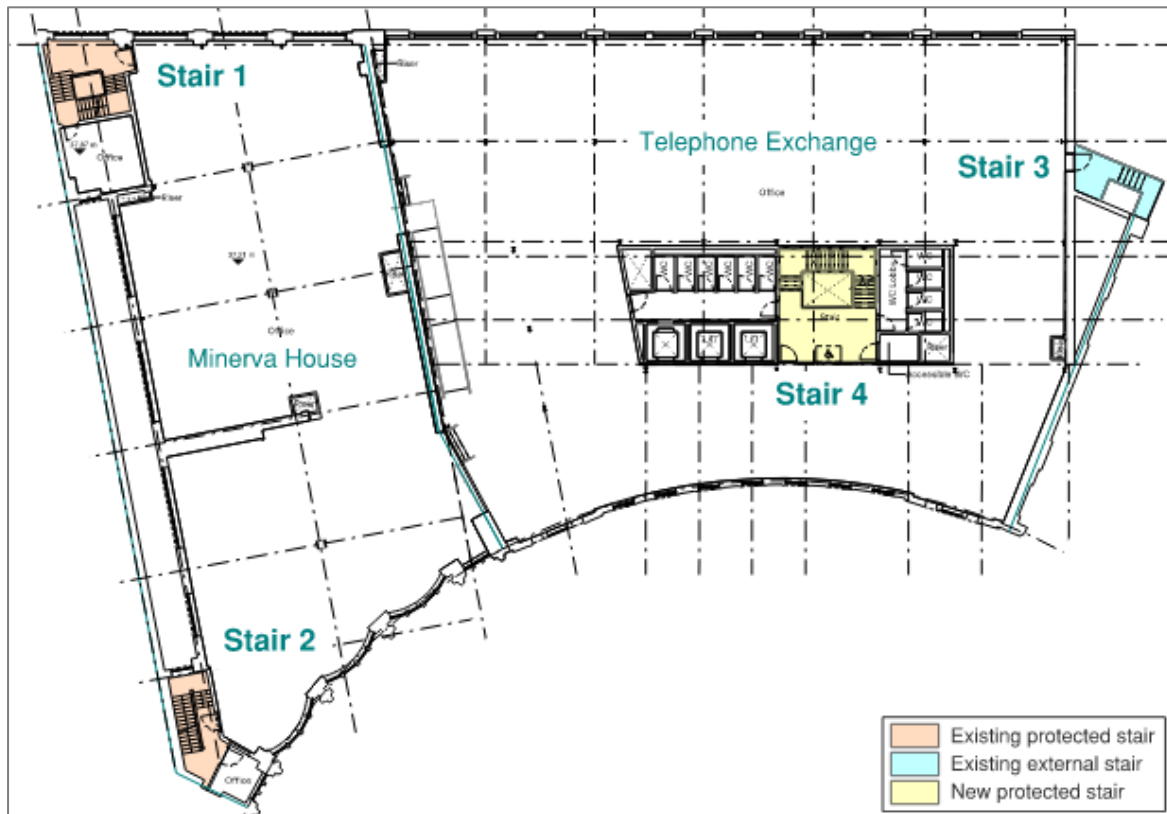
Figure 2: Escape Stairs on the Second Floor
